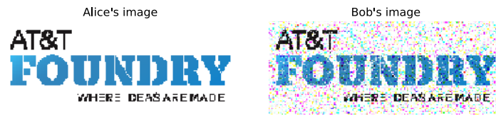
Figure E.8: Results of Program E.6, showing Alice’s original image (left), and Bob’s received image (right). Bob applies no correction for attenuation errors, replacing dropped qubits with bit pairs of (0, 0).
