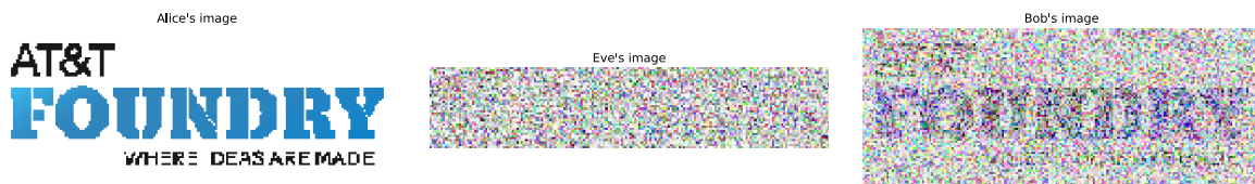
Figure E.10: The results of the simulated interception attack simulated by Program E.7. Since Eve only has access to half of the entangled |AB\rangle state, she recovers only random noise, and Bob’s image is half-corrupted, alerting him to the presence of an eavesdropper.
